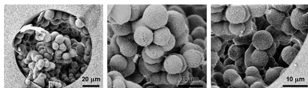
Figure 4. Scanning electron microscopy images of polymer 4 prepared in situ in a fused-silica mold (100 \mu\text{m} ID) with pendant vinyl groups: left, cross-section; center, bulk region; right, wall region.
